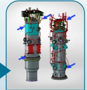
Piping, valves, sensors & cables to pressure vessels
