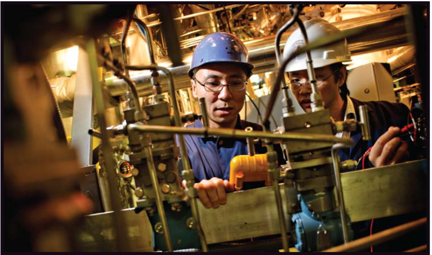
Nuclear scientists YuQuang Li (left) from China's State Nuclear Power Technology Company and Professor HanYang Gu of Shanghai Jiaotong University calibrate instruments for a test of OSU's scale-model reactor.
